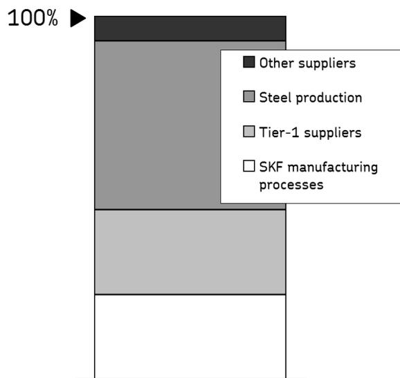
**Fig. 4.** Contributions to global warming from manufacturing a bearing unit (cradle-to-gate).
