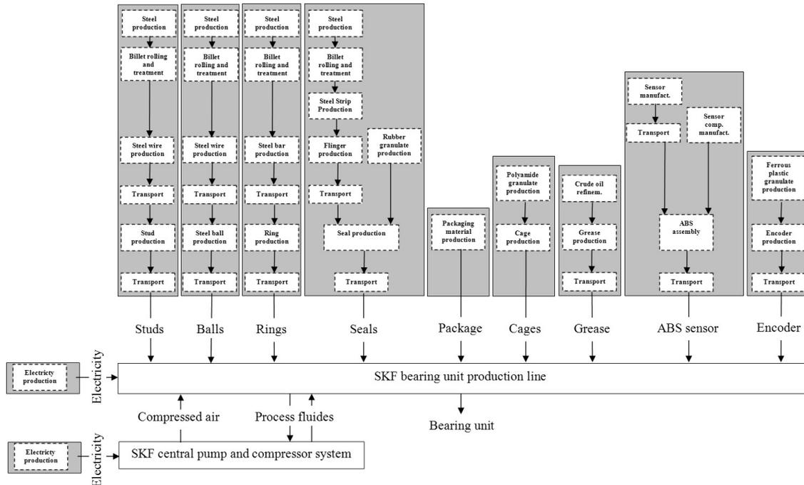
**Fig. 8.** LCA modelling used in Rinde [71] to calculate the LCA factors of components and electricity supplied to the SKF production line. Each grey box represents a system modelled using LCA to calculate the environmental consequences of a component or electricity input to the SKF production line.
