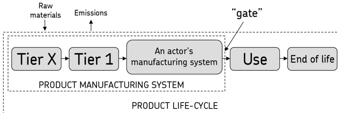
*Fig. 3. The complete product life cycle extending from “cradle to grave”. The product manufacturing system includes the actor’s manufacturing system and its suppliers delivering directly to the actor (i.e. tier 1) all the way up to the very beginning of the value chain (i.e. tier 2,...,x).*
