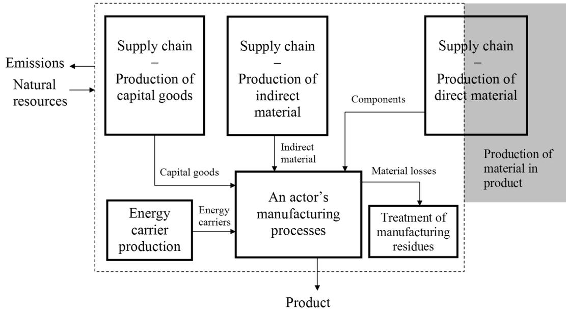
**Fig. 6.** System boundaries, represented by dotted lines, when relating environmental consequences to an actor's manufacturing processes. The supply chain production of capital goods, direct and indirect material, and energy carriers includes all upstream processes required for production. The part corresponding to the material in the product is partitioned away from the processes for producing direct material.
