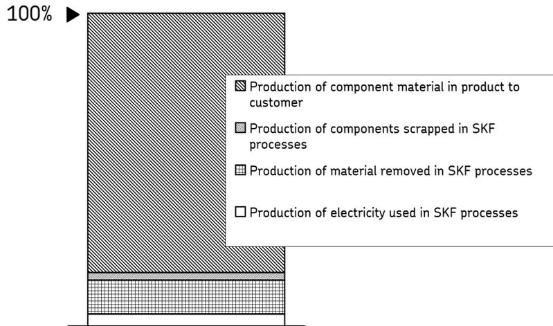
**Fig. 5.** Contributions to global warming from manufacturing a bearing unit, presented relating cradle-to-grave environmental consequences to SKF processes. The same data and system boundaries are used here as in Fig. 4.
