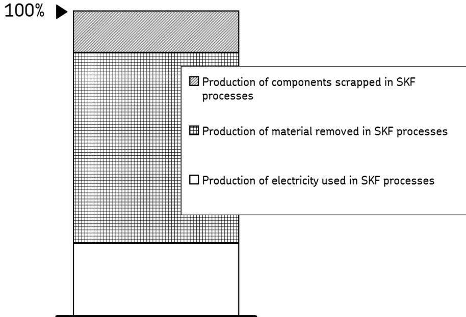
*Fig. 7. Contributions to global warming from SKF manufacturing processes, with system boundaries according to Fig. 6.*
