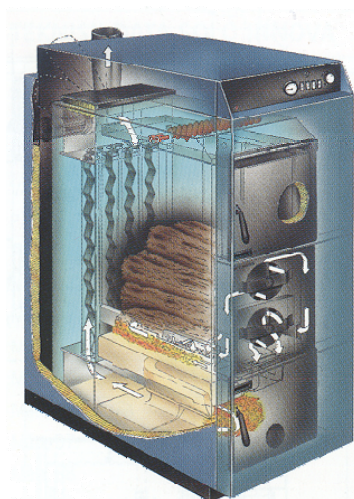
Figure 15: Cross-section of the Baxi Solo Innova wood boiler (Baxi AB 2005).
