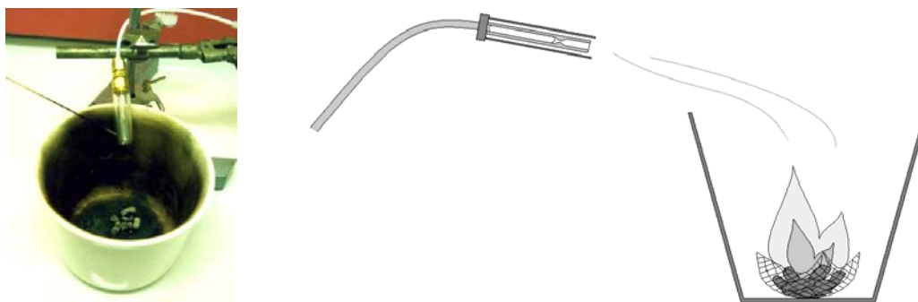
Figure 11: Photo and schematic illustration of the combustion and sampling during studies of organic compounds ( \geq 6C ) on a laboratory scale (I).
