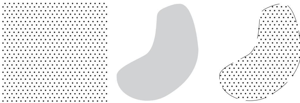
Figure 3.1. Illustration of lattice truncation. Left: a lattice \Lambda , Center: a shape S , Right: the resulting lattice quantizer C .
